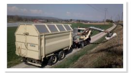
Grass Mower and Grass Container help you cut, collect and remove vegetation from road and rail. Eco Rail technology merged with our partner Müller Technologie AG, gives you robust and flexible mowing and suction technology.
