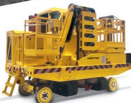
Using the key concepts of the Elan C, the **Elan D** offers a reach of work unparalleled in the category of compact self-propelled machines. Its far-reaching basket (13 m height, 6 m outreach) allows work through 180°, its cabin and new generation of controls offer unique ergonomics and performances. Its flexibility is also increased thanks to his work in road mode.
