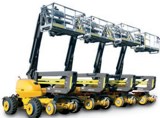
Working on 5 continents, the **SKY W16** is the reference rail/road basket (MEWP). Born from the close collaboration between NEOTEC and MANITOU, it is a totally "RAILED" basket with its vest of class NEOTEC hi-rail axles and the optimal elevation performance with its 400 kg of payload. Made for rail, it offers great flexibility on rail networks, here and elsewhere.
