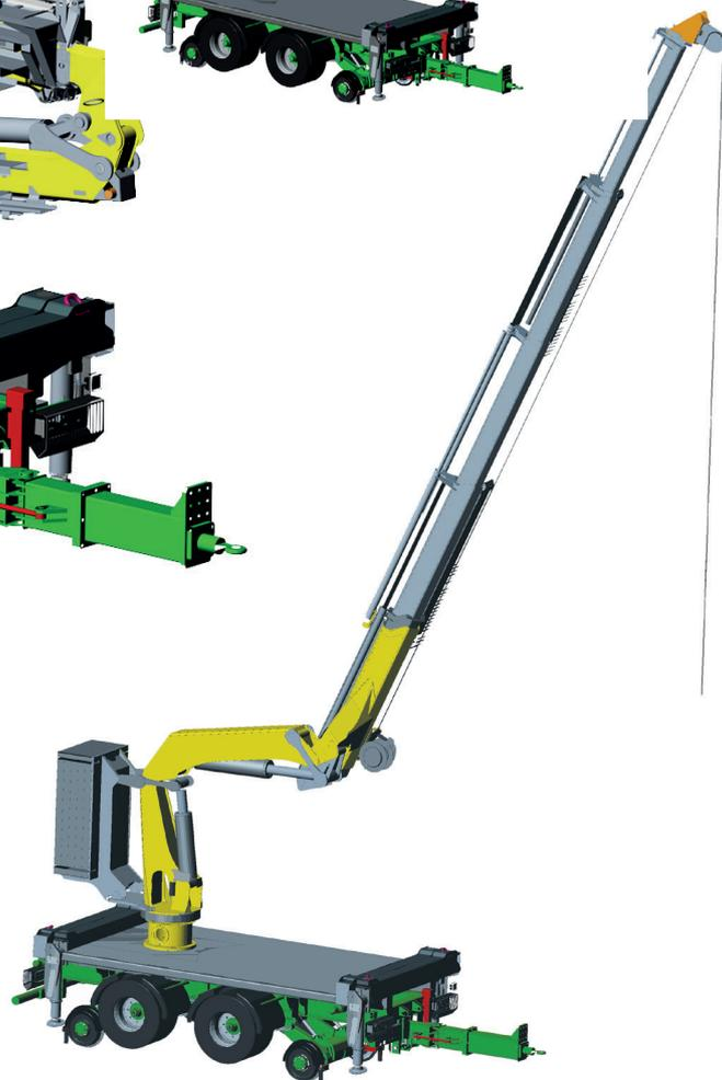
Innovative machine concept for excavators to expand your application range when handling building material, accessing platforms, inspecting bridges, etc.
