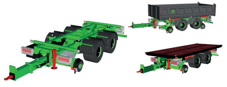
Double-axle, heavy duty trailer flexible for use on road and rail. This chassis can be combined with all Eco Rail accessories, for maximum flexibility during the work shift.
