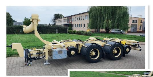
This double-axle, heavy duty trailer is adapted for road registration. Eco Rail multi gauge axle system gives maximum flexibility in different railway systems.
